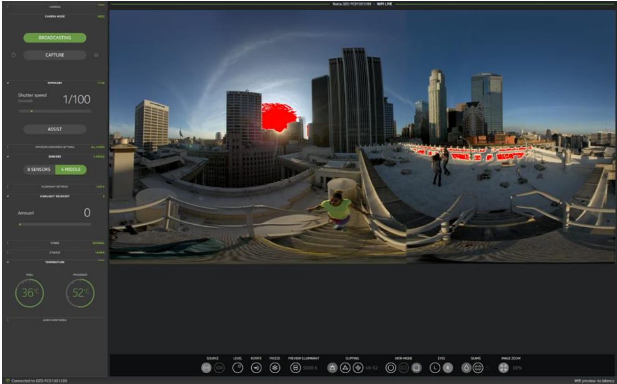
Before adjusting the Highlight Recovery. The red pixel clip false color overlay provides an indication of overexposed zones.
