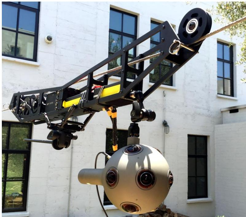
The OZO mounted on a cable cam. This support creates consistent and linear movement.
